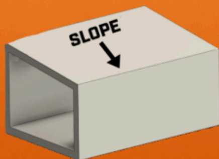
1/2" PER FOOT SLOPE FOR WATER RUNOFF
